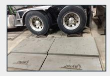
The engine testing was done using a Taylor rolling dynamometer at fixed rpm and load. Stack exhaust emissions were sampled and analyzed using a PEMS (Portable Emissions Measurement System) manufactured by Sensors Inc. EPA test method 40 CFR Part 1065 was used to measure engine fuel consumption to eliminate any influence of extrinsic variables such as wind and rolling resistance, driving style, and terrain.
